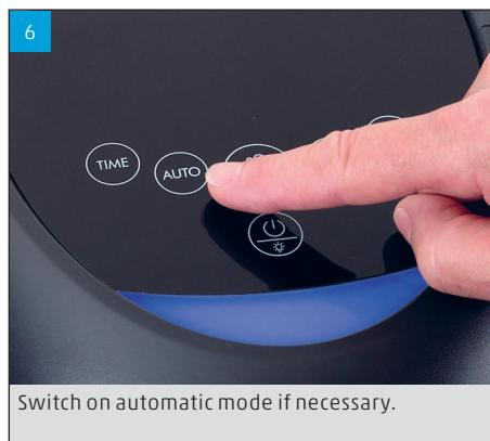
Switch on automatic mode if necessary.
