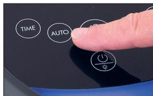
3. To exit automatic mode and switch to manual mode, tap the button for the **performance level**. Each time you tap, you switch between the performance levels: **I > II > III > I**
