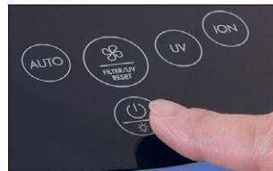
6. Press and hold the button for the performance control for about 5 seconds until the UV warning signal on the display goes out.
